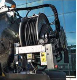
High-pressure reel for large hose capacities
