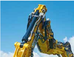
Two-piece offset boom to increase working performance
