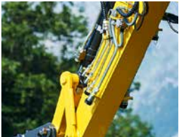
Four-circuit hydraulic system with optional ROTOLINE for the use of power-intensive attachments.
