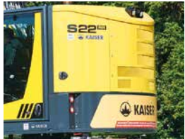
Innovative road-rail excavator in a short-tail design (tail swing radius <math>< 1.57\text{ m}</math>)
