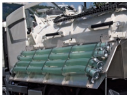
Hose rack - hydraulically tiltable via remote control
