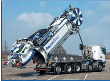
Tipping system and KAISER lock ring.
