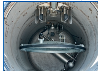
Hydraulically tiltable divider wall. ROTOMAX water recycling system.
