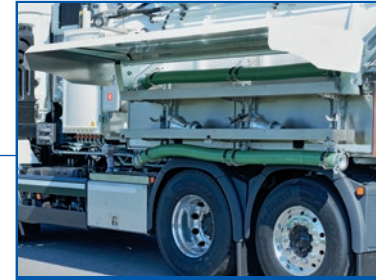
Hydraulic fold-out rack system offering plenty of storage space and flexible use.
