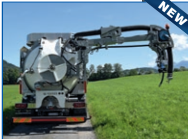
A disconnectable auxiliary hose reel provides enhanced flexibility in the working zone.
