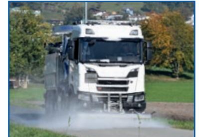
Street cleaning using washing bar with pneumatically actuated swing movement.
