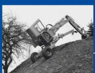
Josef Kaiser Jr. develops a special excavator for use in steep terrain, known as a walking excavator.
