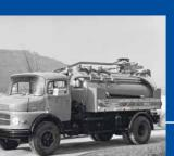
Presentation of the first sewer cleaning vehicle – a sludge vacuum vehicle.
