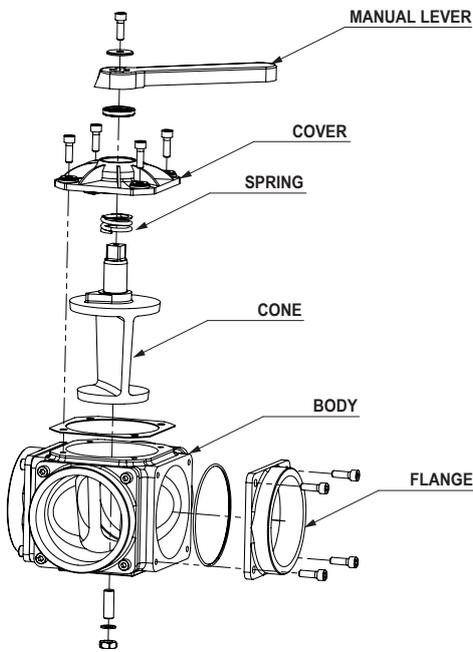
**FOUR-WAY VALVE WITH MANUAL LEVER**
