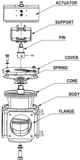
**FOUR-WAY VALVE WITH PNEUMATIC ACTUATOR**
