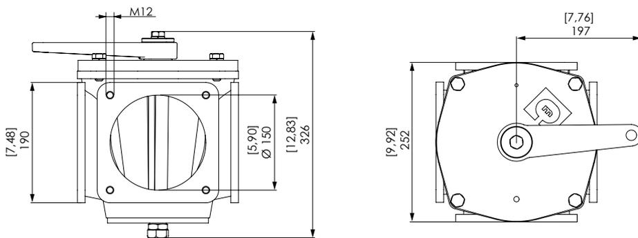
**5" four-way valves with greasing point**
