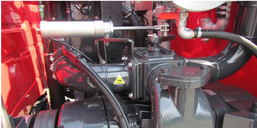
FOUR-WAY VALVES WITH PNEUMATIC ACTUATOR
