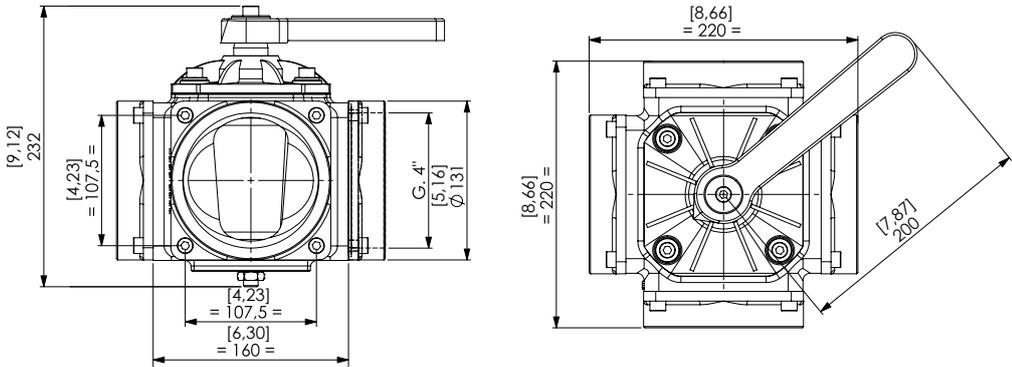
**5" four-way valves without greasing point**
